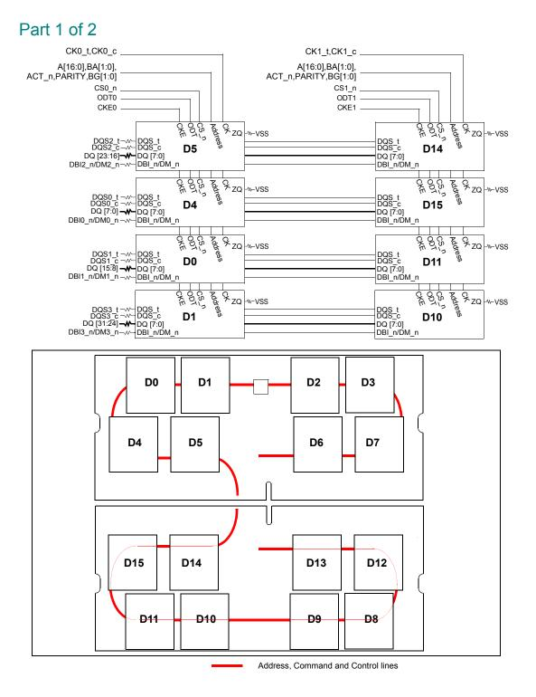
**Note 1:** Unless otherwise noted, resistor values are  $15 \Omega \pm 5\%$ . **Note 2:** ZQ resistors are 240  $\Omega \pm 1\%$ . For all other resistor values refer to the appropriate wiring diagram.
