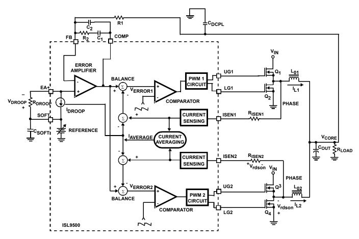
FIGURE 9. SIMPLIFIED BLOCK DIAGRAM OF THE ISL9500 VOLTAGE AND CURRENT CONTROL LOOPS FOR A TWO CHANNEL REGULATOR.
