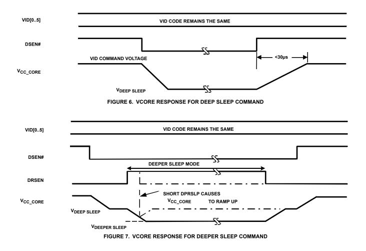
A logic low signal present on DSEN#, with a logic low signal on DRSEN, signals the ISL9500 to reduce the CORE output voltage to the Deep Sleep level, the voltage on the DSV pin, and to operate in diode emulation.
