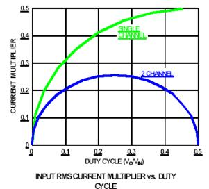
FIGURE 13. INPUT RMS RIPPLE CURRENT MULTIPLIER
