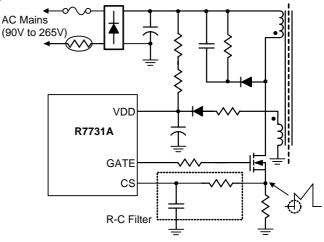
Figure 4. R-C Filter on CS Pin
