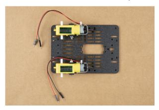
**Note:** Install the motors so the "DAGU robot" sticker is facing out. This will ensure that your JetBot drives forward when following the pictured hookup of the Qwiic Motor driver later in the tutorial.
