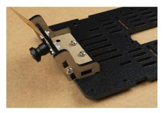
Flip the chassis over & thread two nuts onto the exposed threads of the camera mount hardware.
