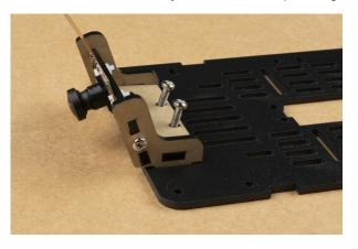
Use your small Phillips head screwdriver to thread the screws through the mounting plates. The chassis kit I got was pretty sung and required me to screw them through.
