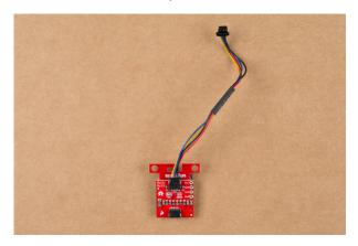
Attach the SparkFun Qwiic Micro OLED to the JetBot Chassis using another Nylon Standoff & 4-40 screw. Attach the 100mm Qwiic cable to the SparkFun Qwiic Motor Driver. Secure the Qwiic Micro OLED by tightening the screw until sung.
