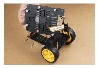
Attach the top plate to the base plate brass standoffs using the four remaining screws from the JetBot chassis kit.
