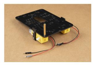
After all standoffs are installed, thread the motor terminal leads through the baseplate as shown. Refer to the photograph of the caster ball assembly to make sure you are using the correctly sized brass standoffs.
