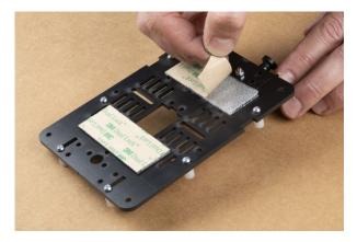
Line up the battery pack as shown to ensure correct orientation of the USB ports & no interference between the battery pack and mounting hardware.
