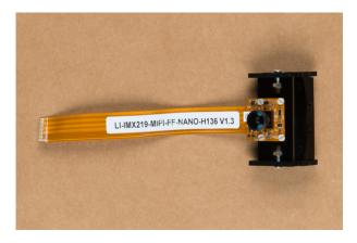
Attach the camera mount & camera to the JetBot Chassis Kit top plate (the unused base plate) using the slightly longer sets of screws and nuts included in the chassis kit (pictured below). Align the plastic tabs on the camera mount to the rectangular cutouts on the front of the chassis top plate. This will result in a sung press fit.
