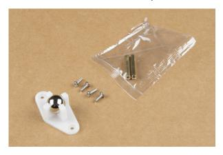
Notice that the brass standoffs used for the caster assembly are slightly shorter than those used for the chassis. The first time you build the SparkFun JetBot, each of these sets of standoffs are packaged together, but it is easy to confuse these once everything has been opened.
