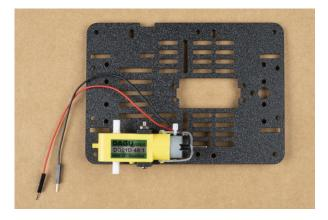
Repeat this process on the other side of the chassis so both motors are symmetric on the base plate.
