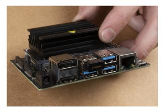
Remove the MicroSD card with the SparkFun JetBot Image (pre-flashed) from the included case & adapter and place it into the MicroSD card slot on the Jetson Nano module. It is easier to do this prior to installing the Jetson Nano Dev Kit onto the chassis and with the Dev Kit upside down as pictured, but you do you.
