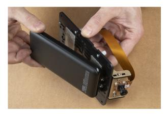
Press firmly on the battery pack to attach the dual lock Velcro interface between the chassis and battery.
