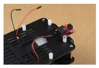
Shown below: Right motor hookup to Qwiic Motor Driver screw terminals.
