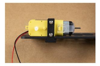
We prefer the shown orientation below that leaves the extra length of the machine screws & nuts on the inside edge of the JetBot.
