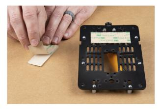
Remove the protective film from the Dual Lock and try not to touch the sticky part.
