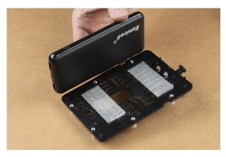
This photo shows how to place the battery pack to not touch the camera mount hardware while not extending too far out the back of the SparkFun JetBot.
