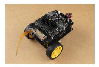
Attach the Leopard imaging camera ribbon cable as shown to the Jetson Dev Kit. This half helix ensures the contacts on the ribbon cable attach to the contact on the Jetson Dev Kit camera connector.
