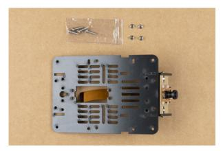
Use the screws to align the holes in the camera assembly with the corresponding holes in the chassis top plate.
