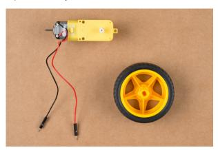
Attach the pair of motors using the long threaded machine screws & nuts included with the JetBot Chassis Kit. The motor will be sandwiched between an internal & external motor mount. Tighten the screws until they are snug.
