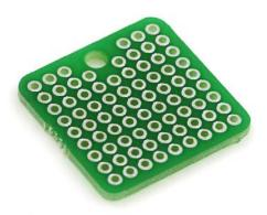
**Description:** This is a very simple but extremely handy, 1" square, single sided perf board. Standard 0.1" spacing with a 4-40 (3mm) hole for mounting. Every three holes are connected with a 20mil trace.
