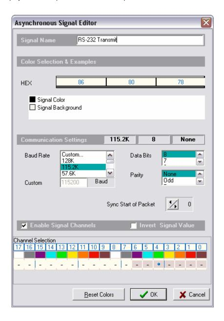
**Signal Name** - Change the text displayed here to help you identify this signal definition. If the name has already been used, it will automatically be appended with a numerical value in brackets (i.e. [2]). The name displayed here will be used in the Waveform Views, searches, tables, lists (if applicable), exports and all menu references.
