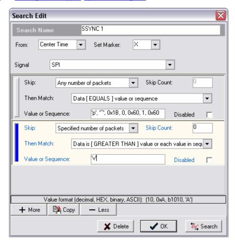
This search type has a group of search terms (or criteria) that is specific to Synchronous signals, and can perform a search sequence by adding additional term groups. Groups can be added by using the Copy or More buttons.
