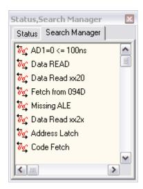
Tabbed windows can be docked just like any normal window. Also, a secondary window can be tabbed with a secondary window that has already been docked. Simply drag the window over the center of the docked window until you see the centered gray rectangle. This will TAB them together at the docked location rather than dock the new window next to the existing window.
