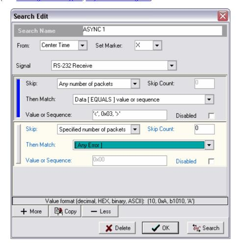
This search type has a group of search terms (or criteria) that is specific to Asynchronous signals, and can perform a search sequence by adding additional term groups. Groups can be added by using the Copy or More buttons.
