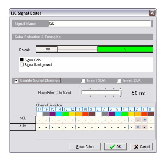
**Signal Name** - Change the text displayed here to help you identify this signal definition. If the name has already been used, it will automatically be appended with a numerical value in brackets (i.e. [2]). The name displayed here will be used in the Waveform Views, Searches, Tables, Lists (if applicable), Exports and all menu references.
