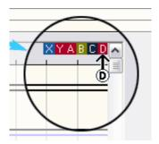
**Dragging** from these flags will bring the marker to the current screen position and make it visible if necessary.
