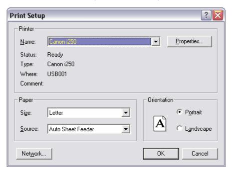
Select a different printer by using the selection box in this window. Available printers can also be selected in the selection box beside the Configure Print Device button if you do not need to access the printers detailed properties. Select the Properties button to access detailed options of the displayed printer.
