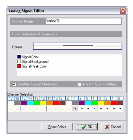
**Signal Name** - Change the text displayed here to help you identify this signal definition. If the name has already been used, it will automatically be appended with a numerical value in brackets (i.e. [2]). The name displayed here will be used in the Waveform Views, searches, tables, lists (if applicable), exports and all menu references.
