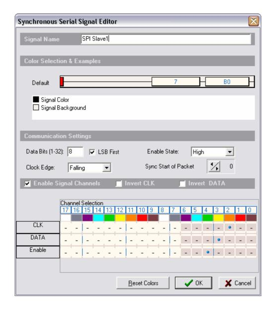
**Signal Name** - Change the text displayed here to help you identify this signal definition. If the name has already been used, it will automatically be appended with a numerical value in brackets (i.e. [2]). The name displayed here will be used in the Waveform Views, Searches, Tables, Lists (if applicable), Exports and all menu references.
