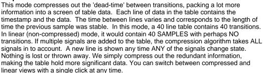
Although compressed mode is the most efficient way to display a signal in tabular form, some people have trouble visualizing the non-linear, compressed time. You can Link a compressed table with other non-compressed tables or with waveform displays to correlate the data to a linear view. This allows BOTH an efficient table view and a linear 'in-context' view.
