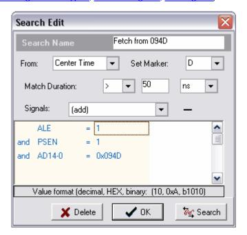
This search type can be used to find a value of one signal or a pattern of values in multiple signals, that lasts for a specified time period.
