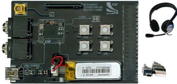
This kit includes all hardware needed to start developing headsets based on the BlueVOX Flash solution, including development PCB, headset and cables and drivers to connect to you PC
