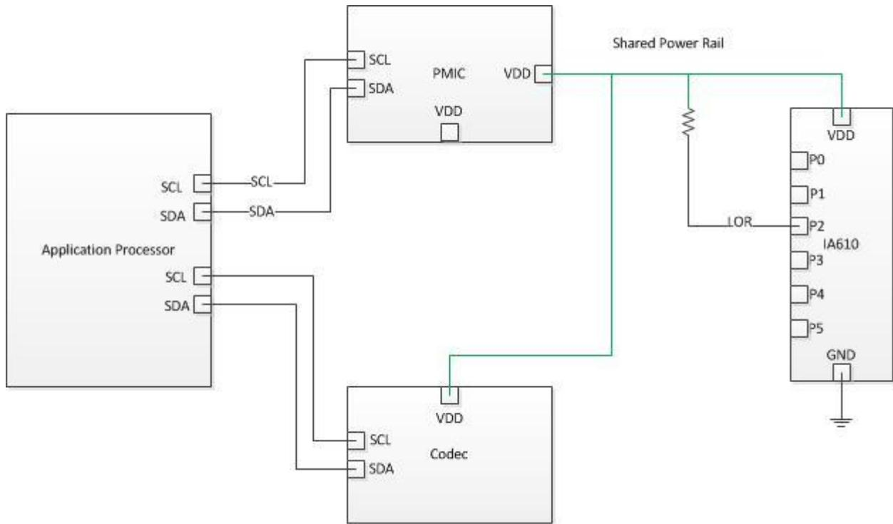
**Figure 8** Latch On Reset with Shared Power Supply
