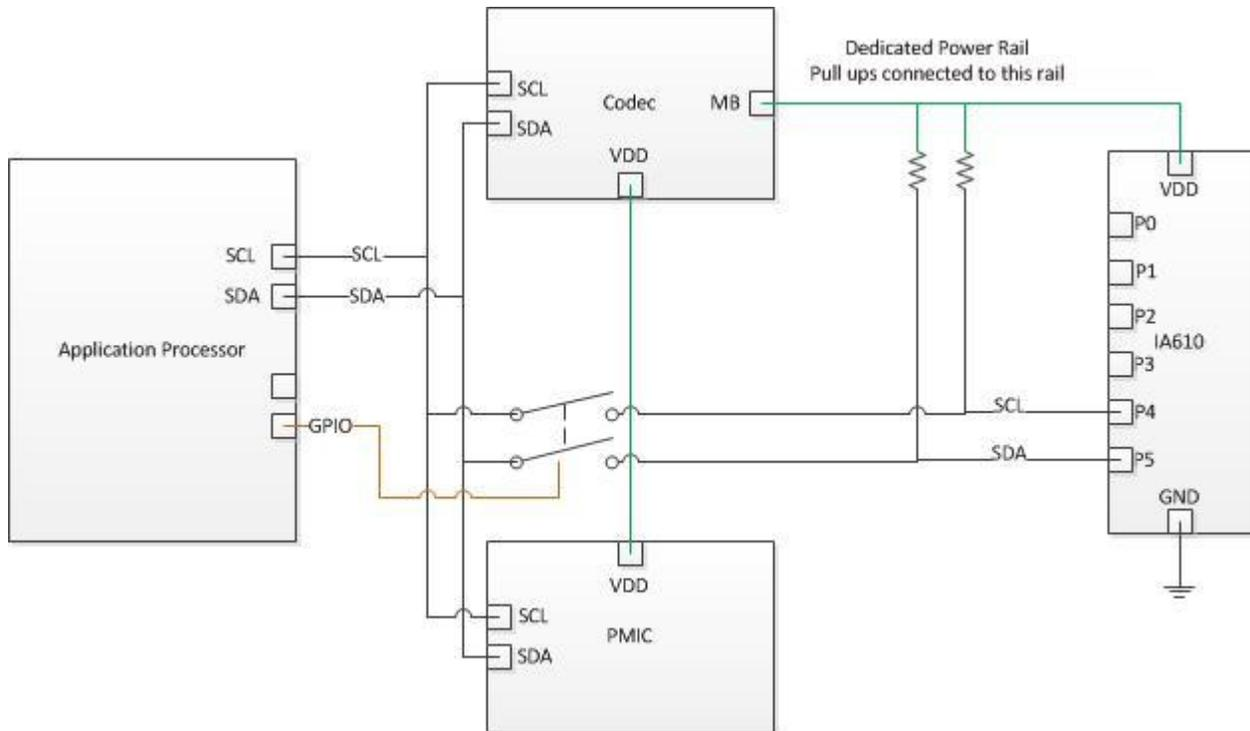
Figure 4 I<sup>2</sup>C Switch Configuration
