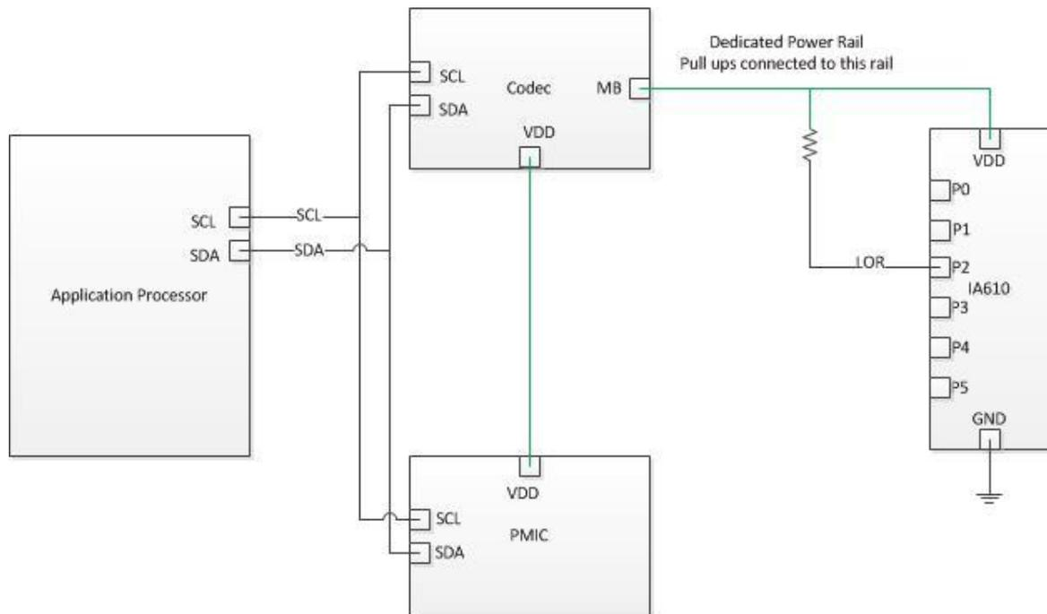
**Figure 7** Latch-On Reset with Dedicated Power Supply
