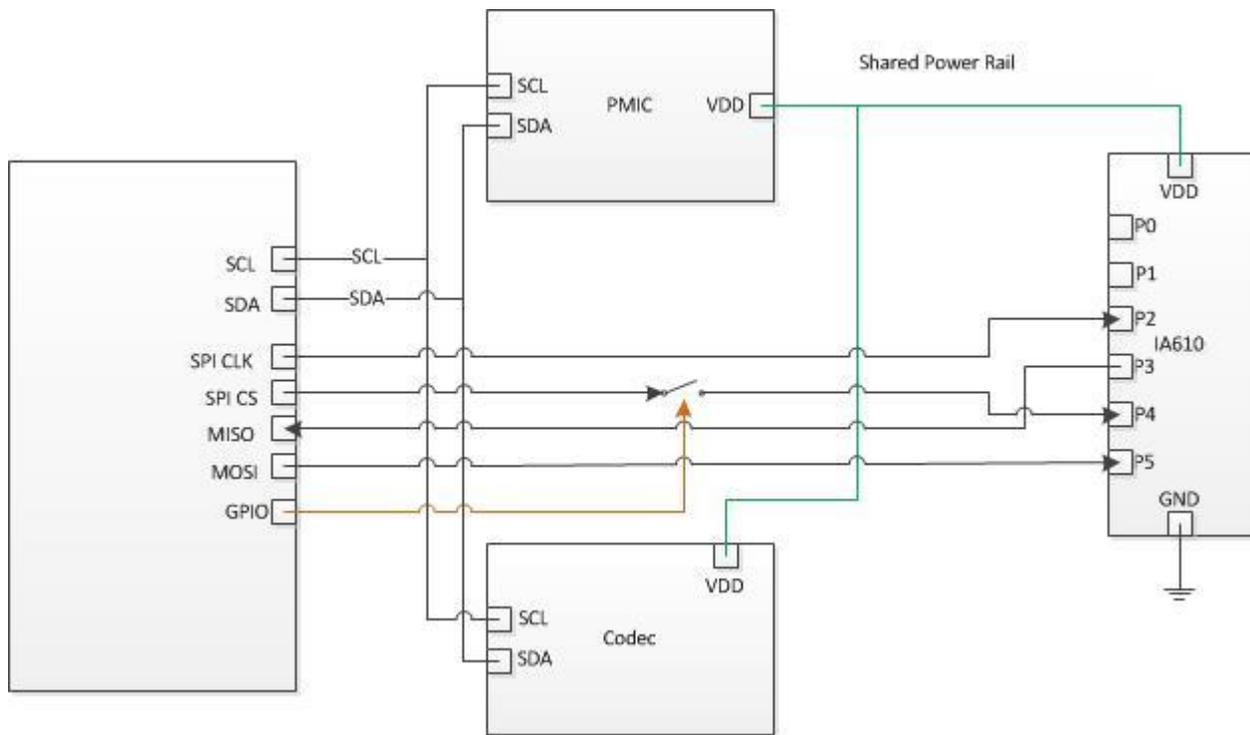
**Figure 6** *SPI CS Isolation Diagram*
