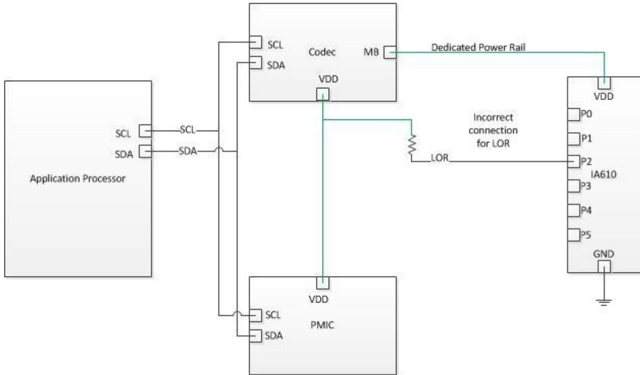
Figure 9 Latch On Reset Incorrect Connection
