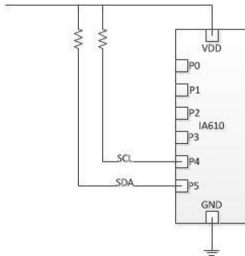
**Figure 1** Pull-Up Resistors Configuration
