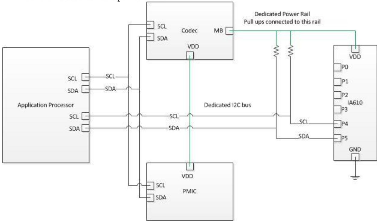
**Figure 2** I<sup>2</sup>C Isolated Configuration
