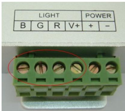
Colour coded screw terminals for LED strip.
