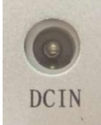
Uses conventional power jack socket as a DC power input from suitable driver (12vDC or 24vDC input)
