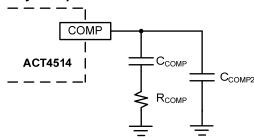
①: C<sub>COMP2</sub> is needed only for high ESR output capacitor
