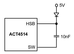
This diode is also recommended for high duty cycle operation and high output voltage applications.
