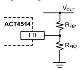
Figure 1 shows the connections for setting the output voltage. Select the proper ratio of the two feedback resistors  $R_{FB1}$  and  $R_{FB2}$  based on the output voltage. Typically, use  $R_{FB2} \approx 10 k\Omega$  and determine  $R_{FB1}$  from the following equation:
