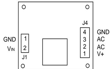
Notes: J1 pin 1: Ground, J1 pin 2: Positive Input  $V_{IN}$
