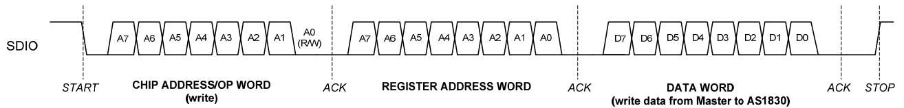
Figure 13 - I 2 C Interface Write Cycle Timing
