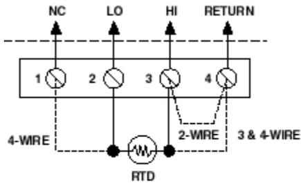
NOTE: 4-WIRE RTD SENSORS MAY BE USED WITH THE 5B34 AS SHOWN. FOR HIGHEST ACCURACY, MODEL 5B35 SHOULD BE USED WITH 4-WIRE RTD.
