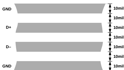
Figure 14. Arrangement of Signal Tracks
