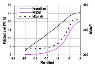
Figure 6. Output Power, PAE, and Drain Current vs Input Power at 30GHz
