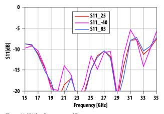
Figure 11. |S11| vs Frequency and Temperature
