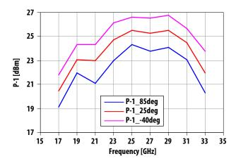
Figure 14. P<sub>-1dB</sub> vs Frequency and Temperature
