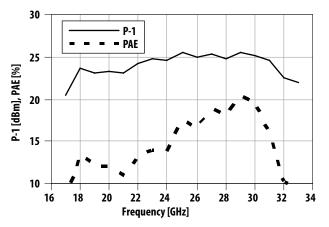
Figure 3. P-1dB and PAE vs Frequency
