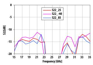
Figure 12. |S22| vs Frequency and Temperature
