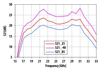
Figure 13. |S21| vs Frequency and Temperature
