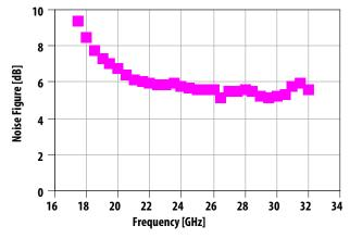
Figure 5. Typical Noise Figure vs Frequency
