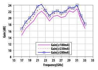
Figure 8. Small signal gain vs Frequency and I<sub>dQ</sub>, (Vds=5V)
