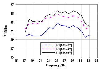
Figure 7.  $P_{-1dB}$  vs Frequency and Vds, ( $I_{dQ}$ =230mA)
