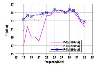
Figure 10. P<sub>-1dB</sub> vs Frequency and I<sub>dQ</sub>, (Vds=5V)
