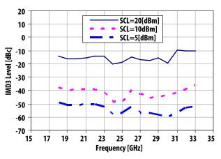
Figure 4. Typical IMD3 vs Frequency (SCL = Single Carrier level)
