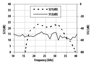
Figure 1. Gain and Reverse Isolation vs Frequency
