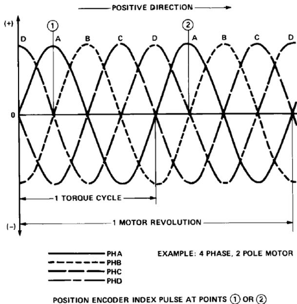
Figure 7. Index Pulse Alignment to Motor Torque Curves.
