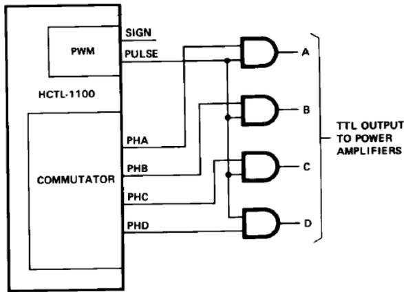
Figure 9. PWM Interface to Brushless DC Motors.
