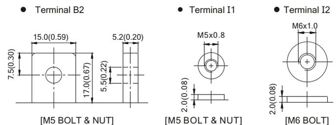
Terminal Hardware Initial Torque:
