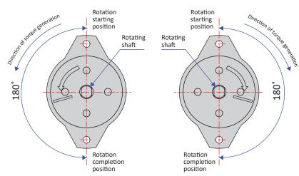
• The damper's working angle is 180° with respect to the attachment flange, as shown to the left. Please determine where to attach it according to your needs. Also, rotating the damper beyond this angle will cause damage to the damper. Please ensure that an external stopper is in place.
