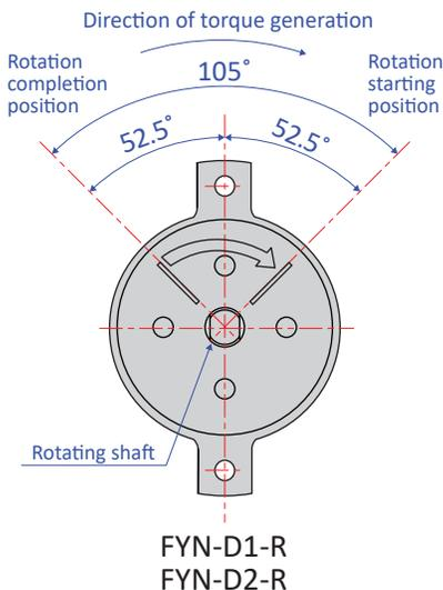
■ The damper's working angle is 105° with respect to the attachment flange, as shown to the left. Please determine where to attach it according to your needs. Also, rotating the damper beyond this angle will cause damage to the damper. Please ensure that an external stopper is in place.
