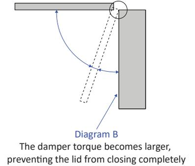
The angle in which the damper torque becomes large can be customized by modifying the inside orifice
