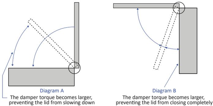
The angle in which the damper torque becomes large can be customized by modifying the inside orifice
