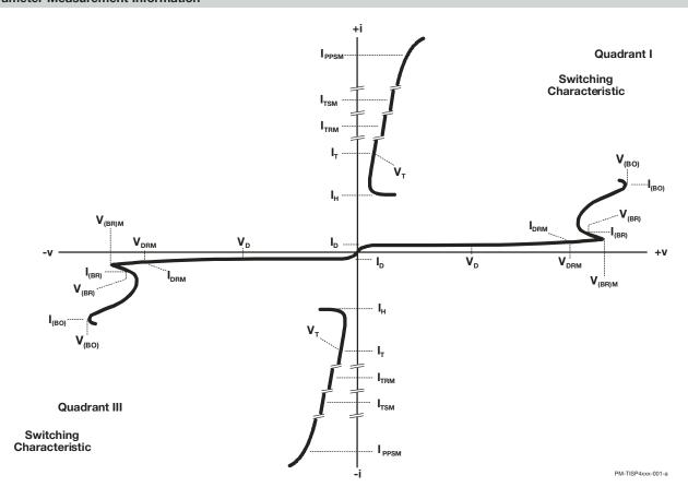
Figure 1. Voltage-Current Characteristic for the Terminals T and R All Measurements are Referenced to Terminal R
