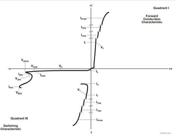
Figure 2. Voltage-Current Characteristic for Terminals T and G or R and G All Measurements are Referenced to Terminal G
