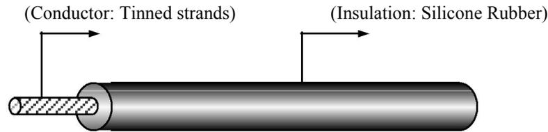
**UL3099 - Silicone Rubber Wire 150°C 300V (16 AWG)**
