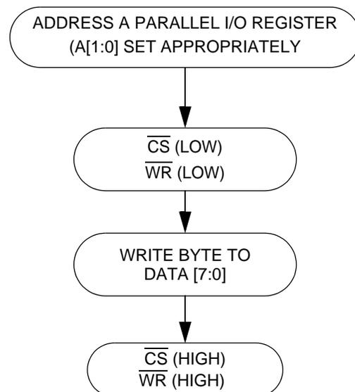
**Figure 24. Intel Mode, One-Byte Write Flow Dia-**
