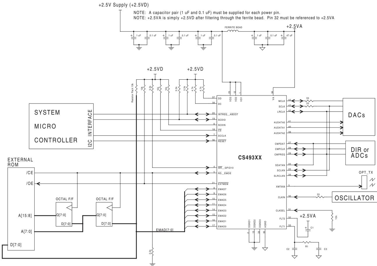
**Figure 14. I<sup>2</sup>C® Control with External Memory**
