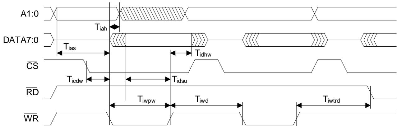
**Figure 4. Intel® Parallel Host Mode Write Cycle**
