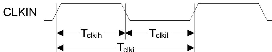
Figure 2. CLKIN with CLKSEL = VSS = PLL Enable
