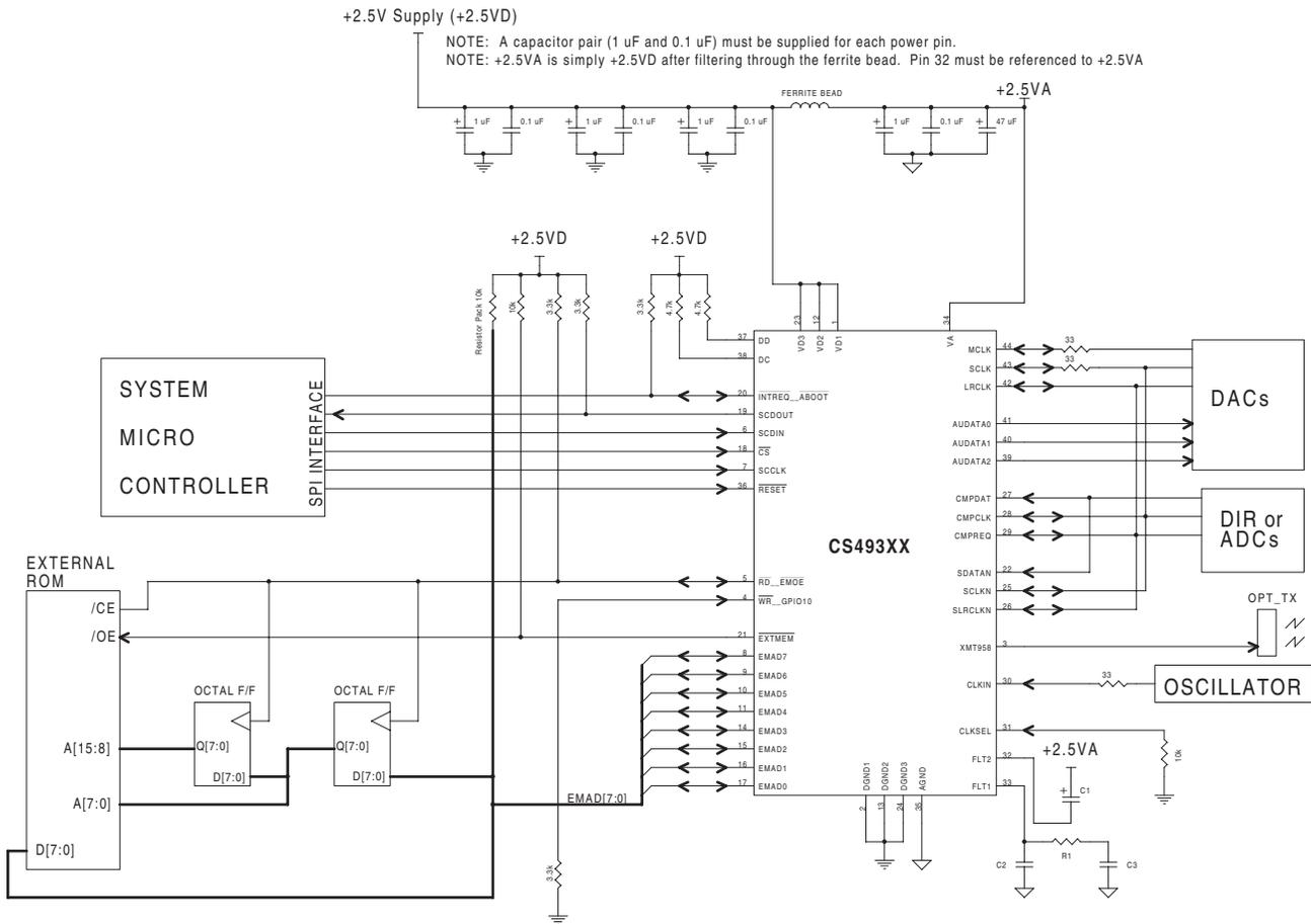
**Figure 16. SPI Control with External Memory**
