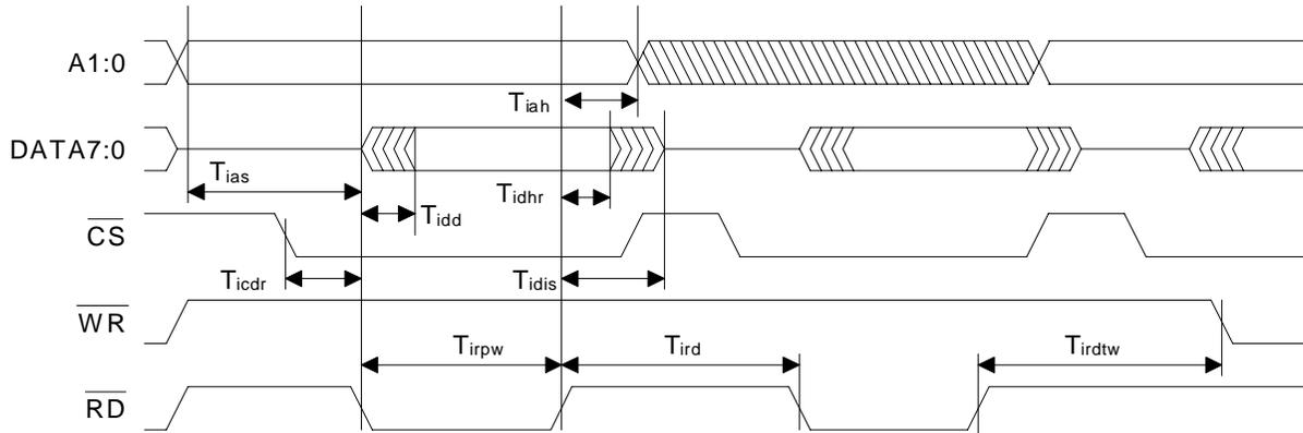
**Figure 3. Intel® Parallel Host Mode Read Cycle**
