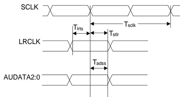
**Figure 12. Digital Audio Output Data, Input and Output Clock Timing**
