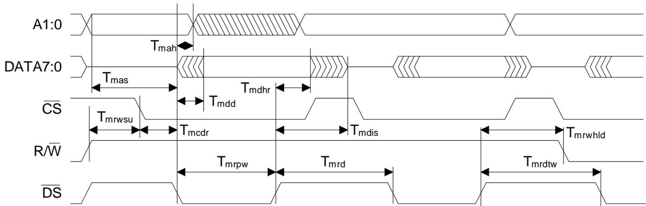
**Figure 5. Motorola® Parallel Host Mode Read Cycle**
