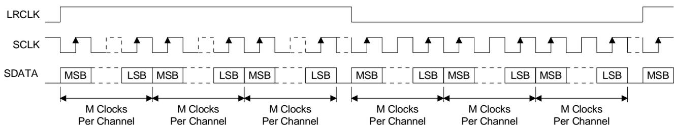
**Figure 45. Multichannel Format**
