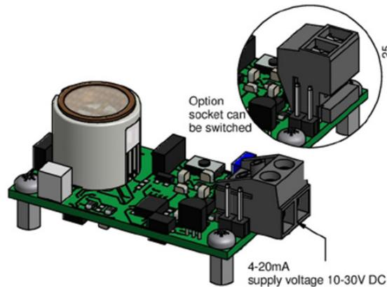
The Gas Sensor Module offers reverse polarity protection, so the power supply can be connected in either direction.
