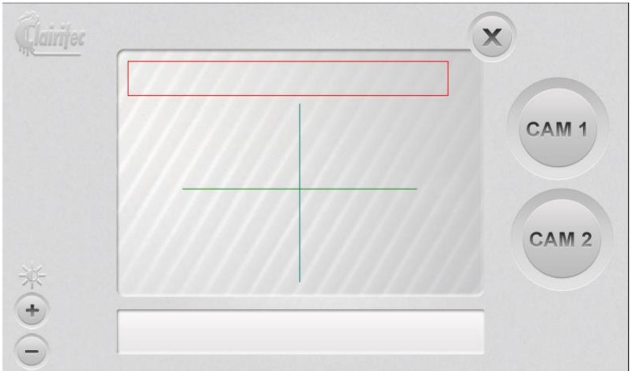
The HMI screen is composed out of 6 touchable buttons, 2 text zones, a red rectangle, and two lines (green and blue). All of these elements have been placed with the HMI Editor of GraphConverter.
