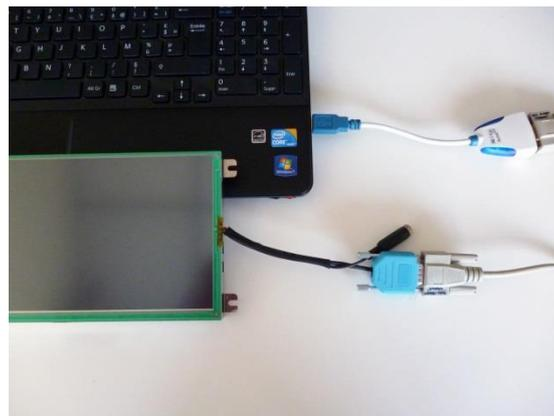
Upon powering up your Intelligent Display, the first image of the graphic library is automatically displayed in the center of the display. The StarterKit contains the logo of Clairitec as its first image.
