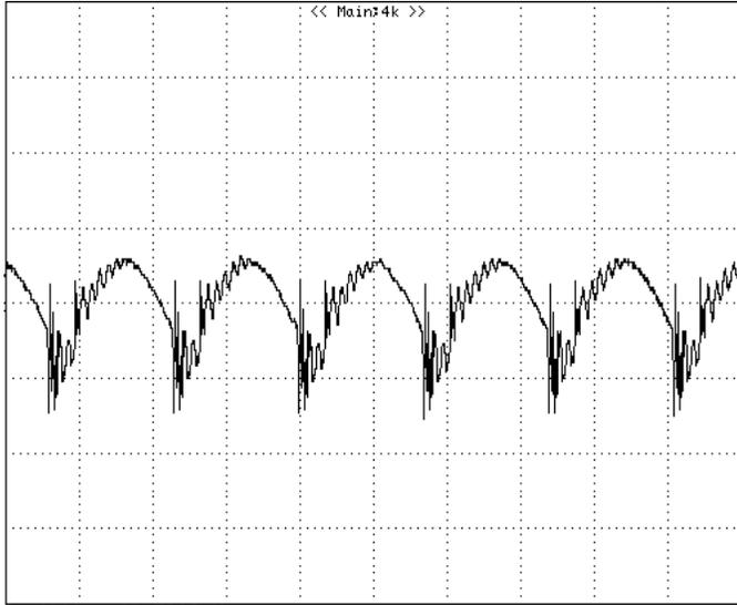
**Figure 14:** Output voltage ripple at nominal input voltage and rated load current ( $I_o=4A$ ) (20 mV/div, 2us/div)
