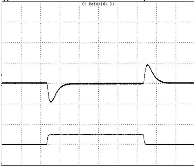
**Figure 8:** Output voltage response to step-change in load current (75%-50%-75% of  $I_o$ , max;  $di/dt = 0.1A/\mu s$ ). Load cap:  $10\mu F$ , tantalum capacitor and  $1\mu F$  ceramic capacitor. Top Trace:  $V_{out}$  (100mV/div, 500us/div), Bottom Trace:  $I_{out}$  (2A/div). Scope measurement should be made using a BNC cable (length shorter than 20 inches). Position the load between 51 mm to 76 mm (2 inches to 3 inches) from the module..
