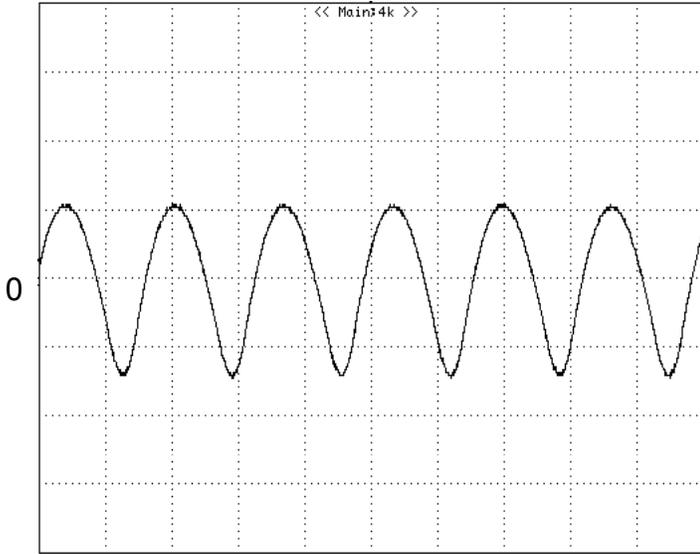
**Figure 11:** Input Terminal Ripple Current,  $i_c$ , at full rated output current and nominal input voltage with  $12\mu\text{H}$  source impedance and  $33\mu\text{F}$  electrolytic capacitor (500 mA/div, 2us/div).
