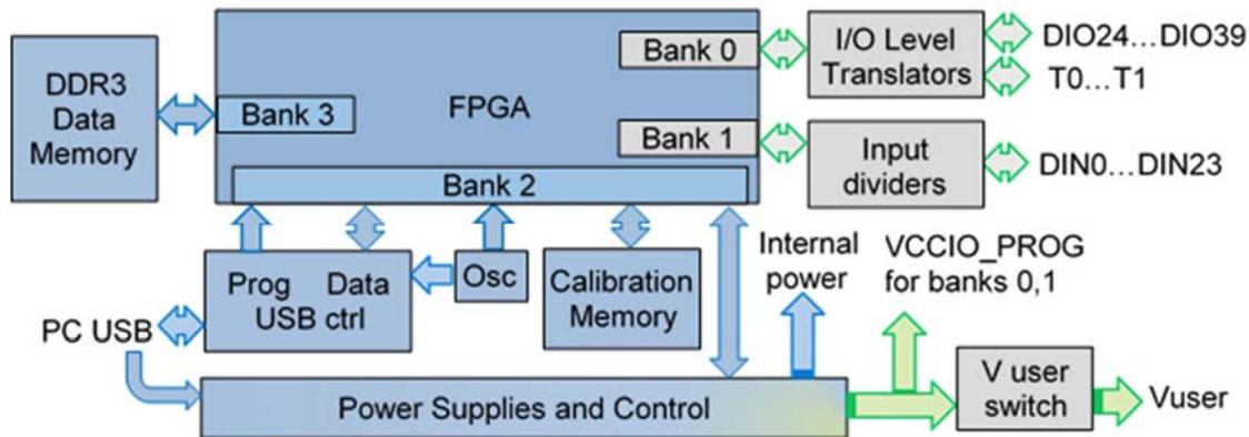
Figure 2. Digital Discovery Hardware block diagram.
