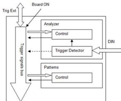
Figure 20. FPGA configuration trigger block diagram.
