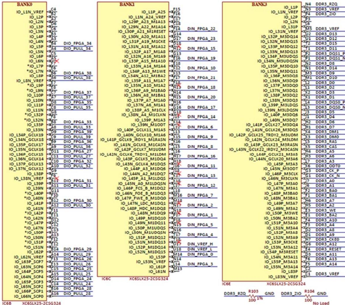
Figure 21. FPGA banks 0, 1 and 3.
