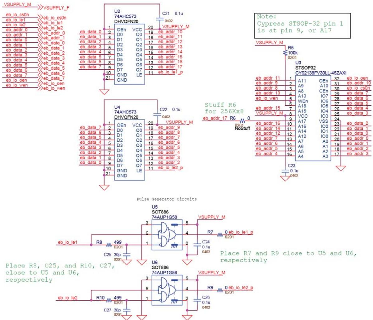
**Figure 7 Eterna Extended Memory Example Schematic (page 2 of 2)**
