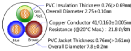
SJT 18AWG×3C (Wire Cross-Section)
