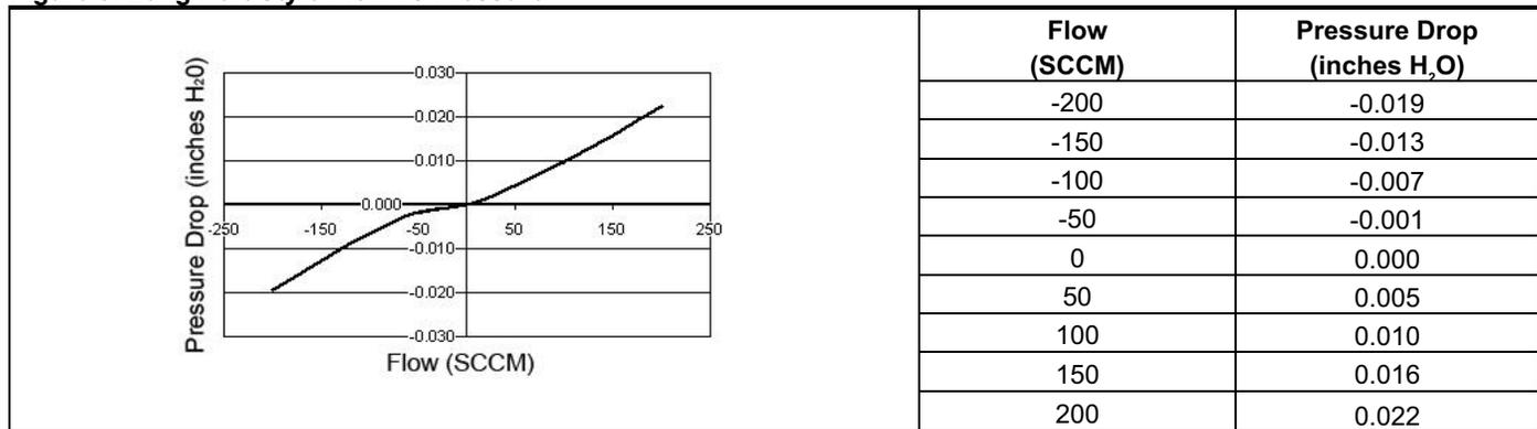
Figure 6. Short Port Style Flow vs Pressure
