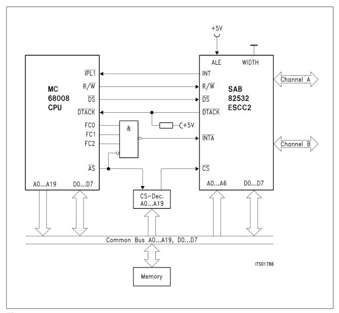
Figure 9 ESCC2 with MC 68008
