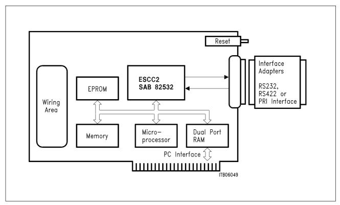
Figure 71 Block Diagram EASY532
