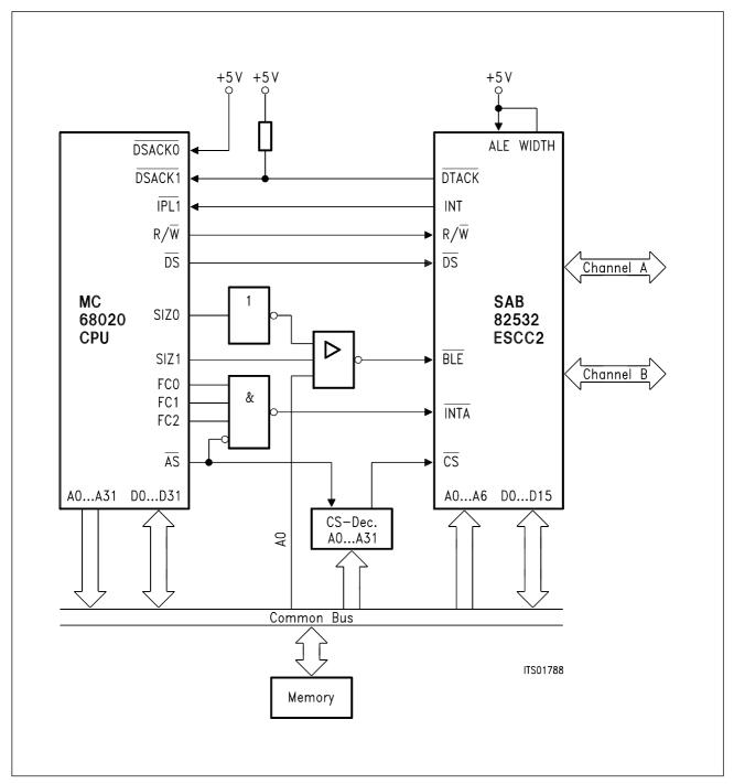
Figure 11 ESCC2 with MC 68020
