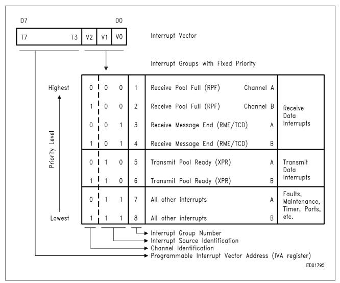
Figure 20 Structure of Interrupt Vector
