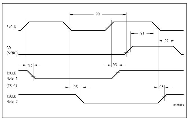
Figure 70 Synchronization Timing
