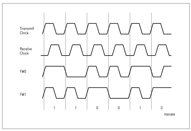
Figure 43 FM0 and FM1 Data Encoding
