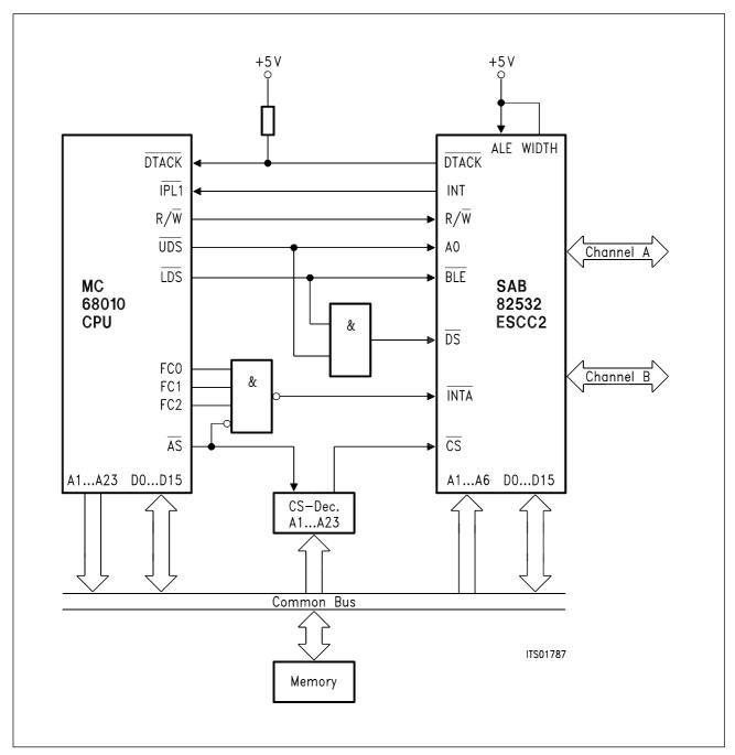
Figure 10 ESCC2 with MC 68010
