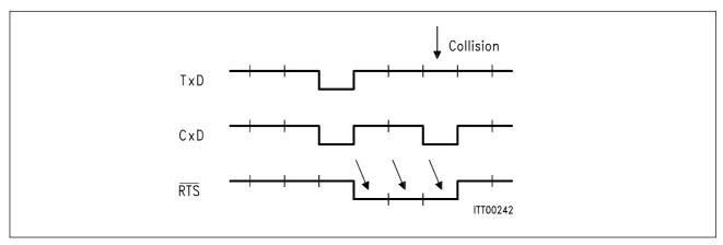
Figure 41 Request-to-Send in Bus Operation
