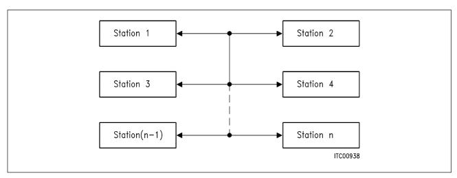
Figure 16c Multimaster Configuration
