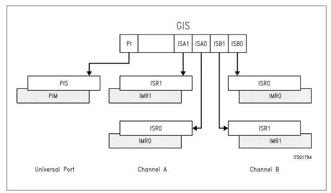
Figure 19 ESCC2 Interrupt Status Registers
