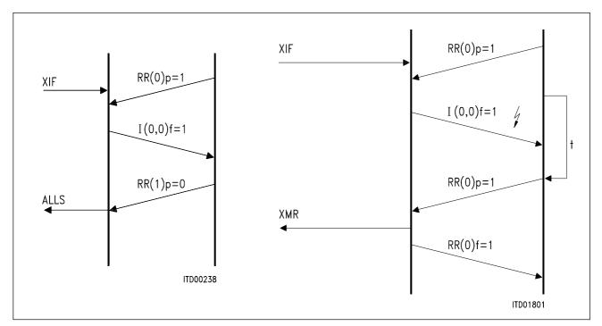
Figure 29a Data Transmission (no error)
