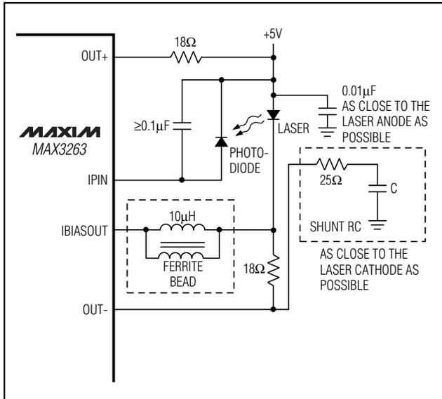
Figure 5. Typical Laser Interface with Bias Compensation
