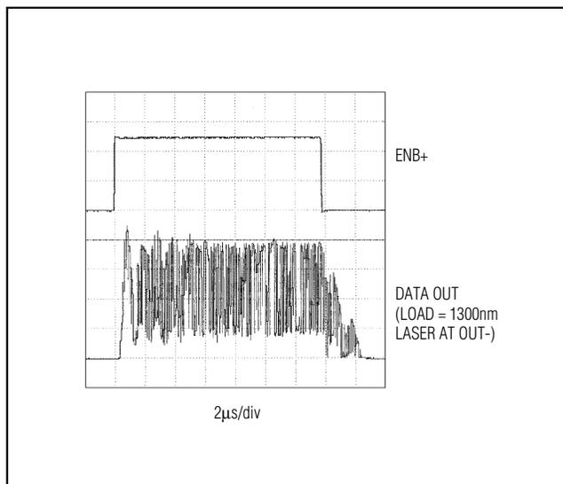
Figure 3. Enable/Disable Operation
