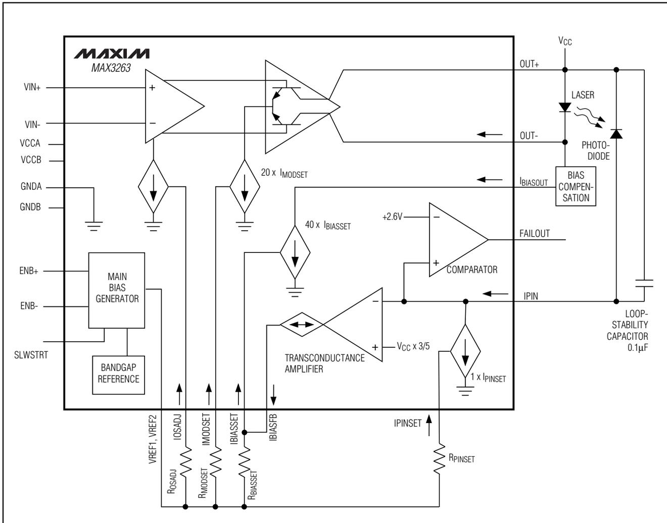
Figure 1. Functional Diagram
