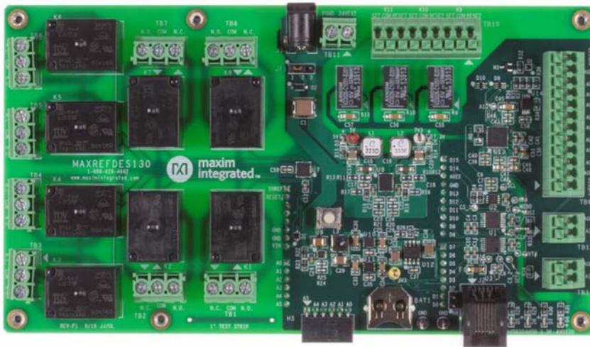
MAXREFDES130# is an Arduino® form-factor shield compatible with ARM® mbed™ and Arduino platforms providing a complete reference for prototyping your next building automation design. This design includes eight 0VDC-10VDC analog outputs, one 4-20mA output, one 4-20mA input, eight nonlatching relays, three latching relays, an RTC, and 1-Wire® master. The MAXREFDES130# works well with one or more of the MAXREFDES131#, the 1-Wire®, Grid EYE® sensor, to make a complete building automation solution.
