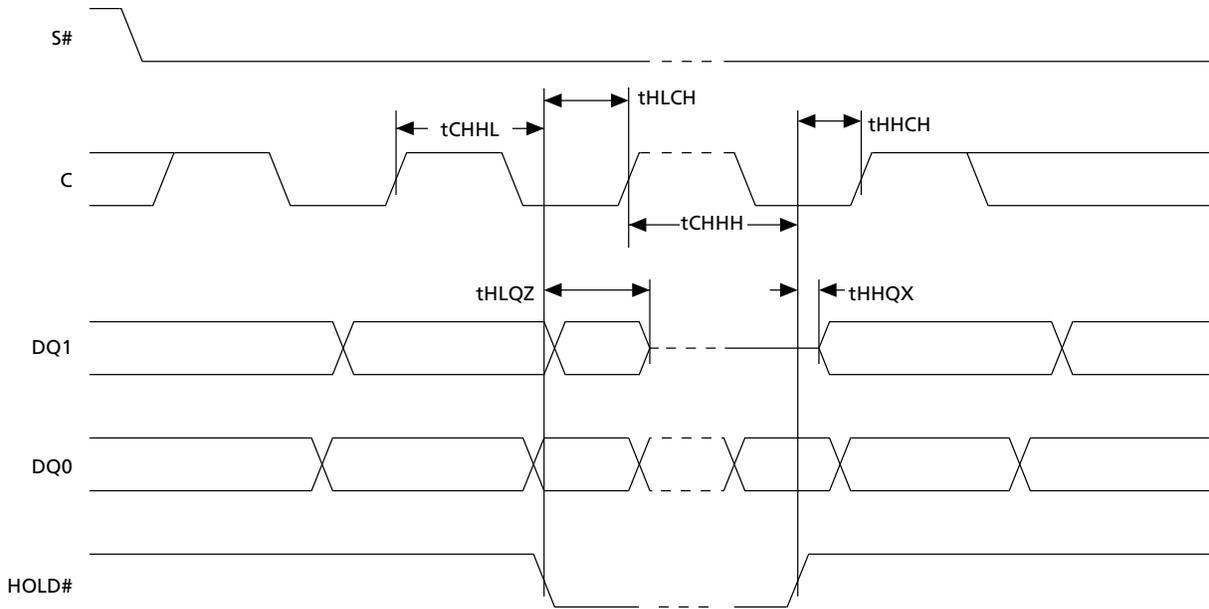
**Figure 27: Output Timing**
