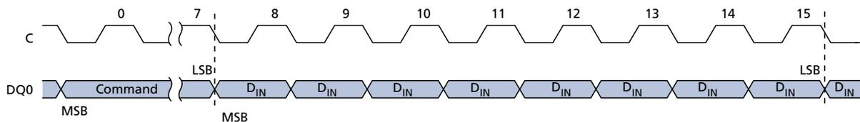
As soon as S# is driven HIGH, the self-timed WRITE STATUS REGISTER cycle is initiated; its duration is  $t_W$ . While the WRITE STATUS REGISTER cycle is in progress, the status register may still be read to check the value of the write in progress (WIP) bit. The WIP bit is 1 during the self-timed WRITE STATUS REGISTER cycle, and is 0 when the cycle is completed. Also, when the cycle is completed, the WEL bit is reset.
