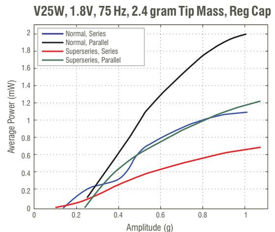
This representative figure shows how the different settings on the EHE004 can be used most efficiently given the vibration profile that this specific energy harvester with this tip mass was subjected to. For lowest amplitude vibrations (in this instance below 0.175 gee)
