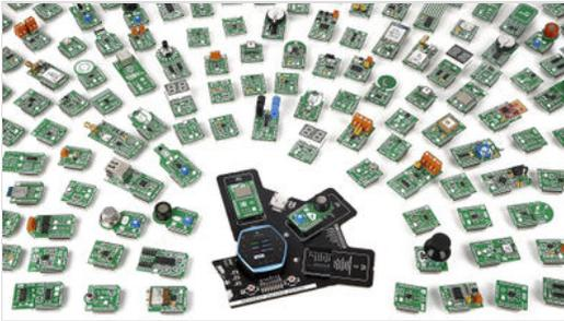
The click board eco-system vastly enhances Hexiwear's potential as a development tool. Hundreds of sensors, actuators, transceivers, displays, ports, encoders and interfaces are available on click boards – add-on boards with a standardized connector and form factor.
