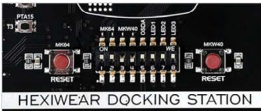
There is a row of 8 configuration switches right under the Hexiwear connector. Switches 1-5 are for setting up the OpenSDA programmer/debugger to connect either to the K64 MCU or the KW4x BLE MCU.
