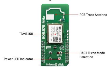
The TCM515U can work in three functional modes: Telegram Reception, Telegram Transmission, Low Power Sleep.
