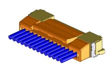
Robust thumb-latch design provides easy operation and two points of positive-lock contact for secure mating retention. The design also provides a strong "click" feeling for mating assurance.
