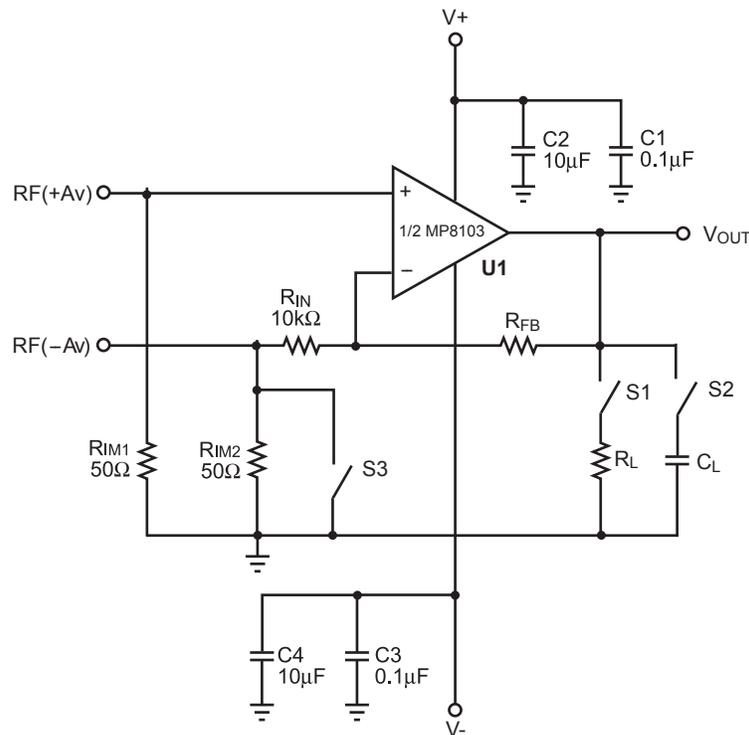
Notes: Close S3 for positive gain. Input signal to RF(+Av) connector.
