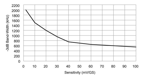
Figure 4. Sensitivity VS Band-width
