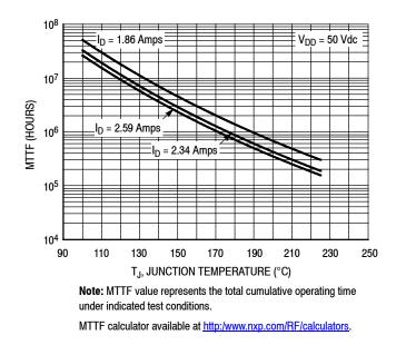
Figure 4. MTTF versus Junction Temperature – CW
