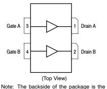
Note: The backside of the package is the source terminal for the transistor.
