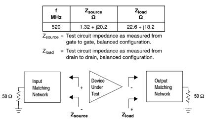
Figure 10. Narrowband Series Equivalent Source and Load Impedance — 520 MHz
