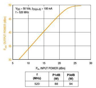
Figure 6. CW Output Power versus Input Power
