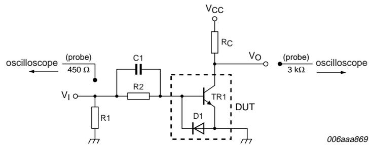
$I_C = 0.05\text{ A}; I_B = 2.5\text{ mA}; R_1 = 50\ \Omega; R_2 = 3\text{ k}\Omega; R_C = 180\ \Omega; C_1 = 1\text{ nF}$
