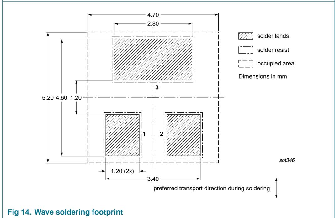
Fig 14. Wave soldering footprint
