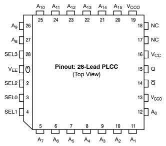
\* All  $V_{CC}$  and  $V_{CCO}$  pins are tied together on the die. Warning: All  $V_{CC}$ ,  $V_{CCO}$ , and  $V_{EE}$  pins must be externally connected to Power Supply to guarantee proper operation.
