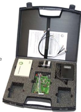
The provided motherboard gives a lot of flexibility during your development process. Easy access to several signals makes debugging very easy and gives you the possibility to connect the evaluation kit with your own application which reduces the development time. Evaluation of the complete NCV7052x family is made very easy by means of the separate daughterboards.
