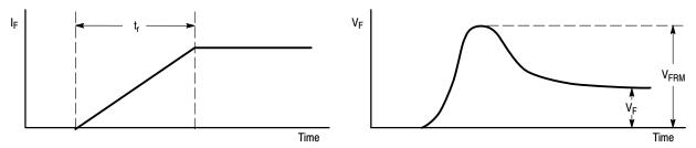
Figure 4. Peak Forward Recover Voltage Definition
