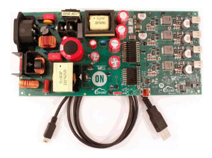
The 4-Port USB-PD Source showcases ON Semiconductor's broad portfolio of USB-PD power solutions, including the FUSB307 PD Port Controller, the FUSB252 HV Protection Switch, and the NCP81231 buck controller. The universal 200W AC/DC supply uses the NCP1399 LLC controller, the NCP1615 PFC, and NCP4305 secondary SR controller providing a highly efficient front-end solution. All ports are 100W capable with a total max system power limited to 200W using our First Come
