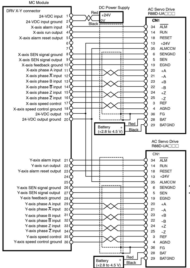
**Note** 1. The terminals marked with asterisks are for use with absolute encoders
