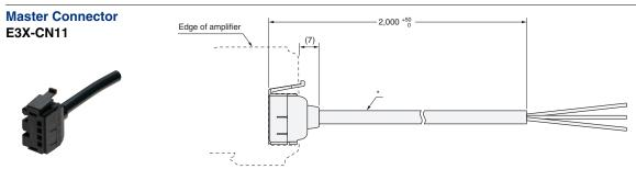
\* E3X-CN11: 4 dia. cable / 3 conductors / Standard length: 2 m (Conductor cross section: 0.2 mm<sup>2</sup> (AWG24), Insulator diameter: 1.1 mm)
