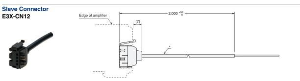
\* E3X-CN12: 2.6 dia. cable / 1 conductor / Standard length: 2 m (Conductor cross section: 0.2 mm<sup>2</sup> (AWG24), Insulator diameter: 1.1 mm)
