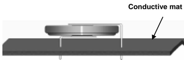
Terminal attached battery installed into a conductive mat had been completely discharged after several days
