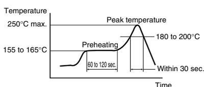
(6) Measure the temperature at the connector surface.
